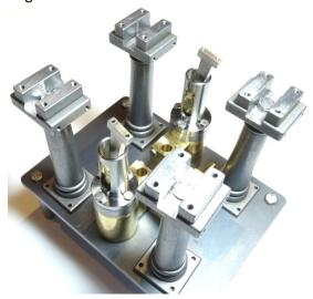
25. Assemble the 2 Top Plates with the Bearing Upper and Lower halves, Main Bearing Support blocks and Single Cylinder Cranks using the M3 30mm setscrews and nuts as shown in the picture. Do not tighen the nuts at this stage.
