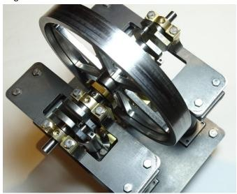
32. The arms of the 2 Cranks need to be set 90 degrees to each other, see pictures. Slightly tighen the 4 grub screws in the Flywheel with the Cranks in this orientation.
