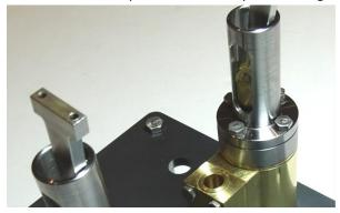
22. Screw the M10 Threaded Rods into the 4 Columns leaving approximately 15mm exposed at the bottom.
