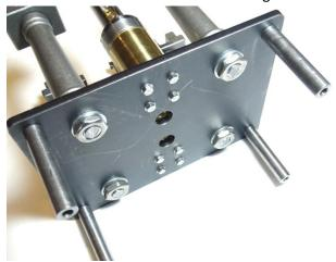
24. Orientate the tops of the Columns as shown in the picture. Do not tighen the nuts at this stage.
