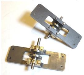
26. Connect the Valves with the Eccentric Rods using M2 10mm setscrews and lock each with a nyloc nut as shown in the following picture. The nut should be left slightly loose to allow free movement of the Valve in operation.
