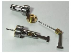
10. Screw the Pistons onto the Piston Shafts. NOTE from the picture the orientation of the Piston.
