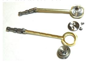
28. Push the Eccentic Wheel/Rod sub-assemblies onto the longer ends of the Cranks as shown in the picture. Do not tighten the grub screws at this stage.
