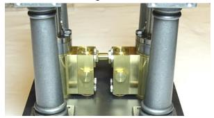
21. Gradually tighten the 8 M3 50mm setscrews from under the Base Plate whilst moving the Connecting Rods in and out. When the M3 setscrews are fully tighened the Connecting Rods should still move up and down freely and be aligned side-to-side as per the picture.
