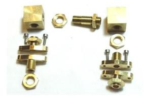
16. Two of the Manifold halves have threaded holes (M2 threads) and the other two have plain holes (2mm). Screw the Manifolds halves that have the threaded holes into the Chests as far as they will go. The Manifolds are locked in place using the ¼" brass nuts.
