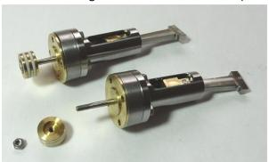
11. Place the Cylinders over the Pistons in the orientation shown in the picture and put the Cylinder End Plate on the end of the Cylinder. Align the holes of in the Mid Plate, Cylinder Plate Inner, Cylinder and Cylinder End Plate.
