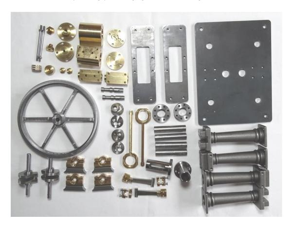
2. Fix the Legs onto the Base Plate using 4 M5 setscrews. The Base Plate surface may be cosmetically better on one side than the other.
