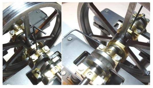
36. The optional Pulley wheel can be place on either side of the engine Crank Shaft and is secured with an M3 grub screw.
