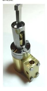
13. Fix the Cylinder sub-assemblies onto the Base Plate fron underneath using 4 M3 50mm setscrews. Do not at the stage tighten the setscrews.
