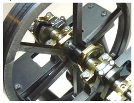
35. The Valve timing is set by fixing the Eccentric Wheels at the angle shown in the following pictures – also show on the Assembly Drawing. The Allen keys show the position of the Eccentric Wheels.
