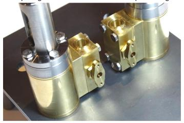
17. Place the 2 M2 setscrews in each of the 2 Manifolds with the plain holes, as shown in the picture.
