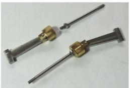
8. NOTE: Usually it is not necessary but the Piston Shaft can be screwed in and out of the Slider to more accurately centralise the "throw" of the piston in the Cylinder.
