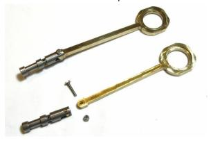
27. Put the Eccentric Wheels and Eccentric Wheel Plates together with the Eccentric Rods using the counter sunk M3 screws, as shown in the following pictures. Then, if not already installed, screw a 3mm grub/setscrew into the Eccentric Wheels which will be used to lock the wheels onto the Crank Shaft.
