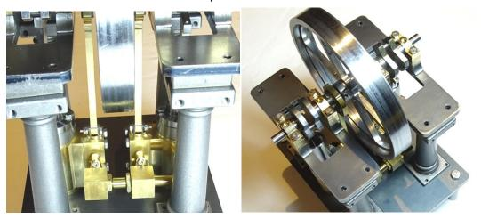
31. Fix the Top Plates to the Columns using the 8 M3 10mm setscrews. Do not tighten at this stage.
