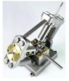
15. If not already in place, insert the 2 nylon piston rings into the slots in the piston and screw the Pistons onto the Piston Shaft. Carefully lock the shafts to the pistons using an M3 nut tightened with a spanner or small pair of pliers.
