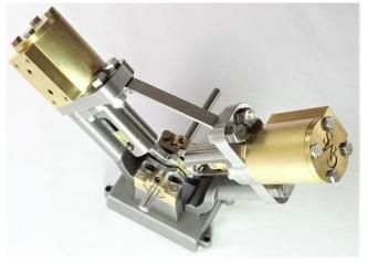
18. If after tightening the Cylinders the engine does not turn over freely try rotating the Cylinder Plates Inner by 90°. Similarly try refitting the Slides/Connecting Rods and their bearings the other way around.
