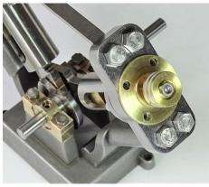
16. Place a Cylinder over the Piston and an End Plate on top of the Cylinders – note the orientation of the flat side of the cylinder as shown on the following picture. Then loosely screw them in place using 4 40mm M3 capscrews.
