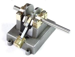
5. Screw the M3 nut onto each Piston Shaft on the longer threaded end. The end of the shaft with the shorter thread is for the Piston.
