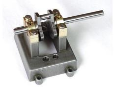
4. Remove the screws holding the connecting rod bearing halves to the connecting rod and place them around the crank shaft as shown in the following picture. Insert and tighten the screws evenly and gradually, rotating the connecting rod around the shaft to ensure the bearing halves locate centrally.
