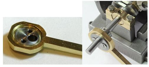
20. Connect the Valves with the Eccentric Rods using M2 10mm capscrews and lock each with a nyloc nut as shown in the following picture.
