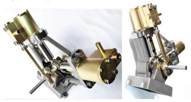
27. If not already in place screw the M3 grub/setscrew into the hole in the Flywheel and push the Flywheel onto the Crankshaft. Tighten the grub/setscrew.
