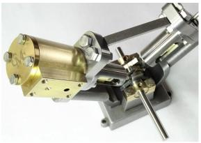
17. Before tightening the 40mm capscrews rotate the Crank Shaft to ensure the Piston can move freely in the Cylinder. There is some tolerance in the Cylinder and Cylinder Plate holes to allow them to be moved into a suitable position to allow free movement of the piston. Then gradually tighten the capscrews. Repeat for the second Cylinder.
