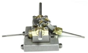
7. Fix the 2 V Twin Side Supports onto the Base using 4 M5 screws. Leave slightly loose. The small plates (20x10mm with 5mm holes) need to be placed between each of the Side Supports and the Base Casting.
