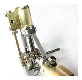
22. Rotate the Eccentric Wheel and Shaft until they are at the correct angle as shown in the following pictures with the Allen/Hex key inserted in the grub screw in the Eccentric Wheel – Piston is at the top of the Cylinder.
