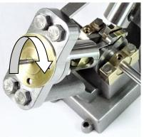
19. Put the Eccentric Wheels and Eccentric Wheel Plates together with the Eccentric Rods loosely using the counter sunk M3 screws. Slide the Eccentric onto the crank shaft to ensure the wheel and plate aligns before tightening the screws, as shown in the following pictures. Then if not already in place screw a 3mm grub/setscrew into the Eccentric Wheels which will be used to lock the wheels onto the Crank Shaft.
