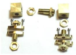
24. Screw the 2 Inlet Manifolds that have threaded holes into the remaining Chest inlet holes.Use the ¼" brass locking nuts to fix the Manifolds in position.NOTE: the red fibre washers are no longer included as they are not really of benefit.
