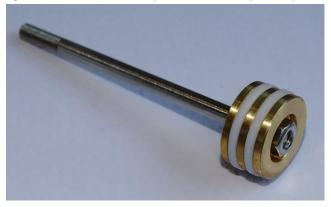
3. Insert each Piston Shaft into a Cylinder Plate Inner and push the Packing Nut onto the shaft and screw into the Cylinder Plate Inner. Screw an M3 nut onto the end of the Piston Shaft.
