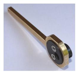
13. Connect each Valve with the Eccentric Rods using an M2 10mm cap screw and lock with a nut as shown in the following picture. The nut should be on the same side as the grub setscrew side of the Eccentric Wheel. If an M2 nyloc nut is included in the kit this can be used instead of a plain nut. Cut or file the cap screw to length as needed.
