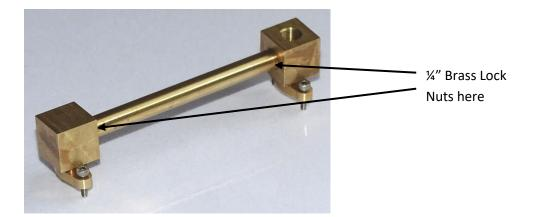
30. Place the Inlet Manifold/Connector subassembly on the Manifolds already installed on the Chests, aligning the Manifold holes to allow the cap screws to go through.
