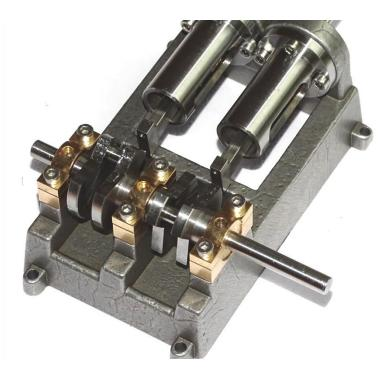
9. One side at a time, place the Connecting Rod Bearing halves and Keep around the Crank Shaft as shown in the following picture. Insert and tighten the cap screws evenly and gradually using the 1.6mm hex/allen key, rotating the connecting rod around the shaft to ensure the bearing halves locate centrally.
