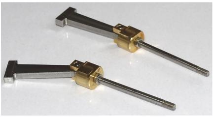
6. Push each Piston Shaft/Tube Slider into a Slider Tube.
