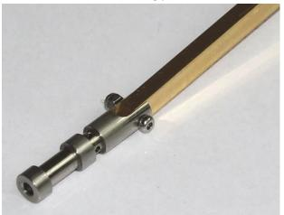
20. Push the 2 Eccentric Wheels on to the 2 ends of Crank Shaft, don't tighten the grub/setscrews yet.
