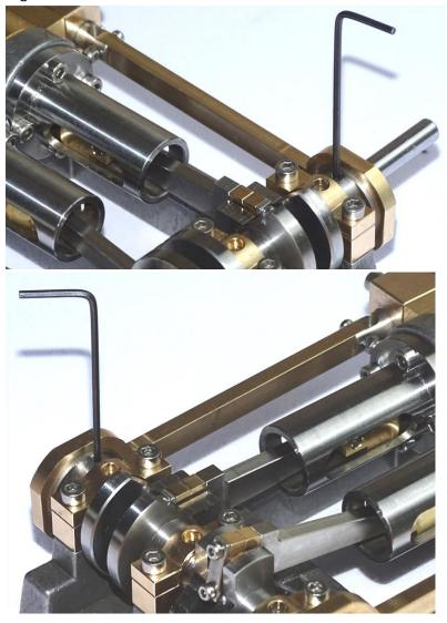
23. The steam inlets can be on top or bottom of the engine Chests. If, as in the following photos, the inlet is on top, screw the 2 Chest Plugs into the holes on the bottom of the Chests. PTFE tape or fibre washers can be used to seal the Chest Plugs if needed. NOTE: The RED Fibre washers are not now included.
