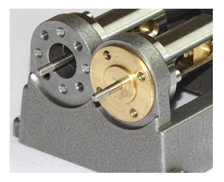
13. Install 2 Piston Rings on a Piston if not already in place, then screw the Piston onto the shaft and lock in place with an M3 nut using a 5.5mm socket spanner or small pliers. Be careful not to damage the Piston Rings when tightening the Piston/nut.
