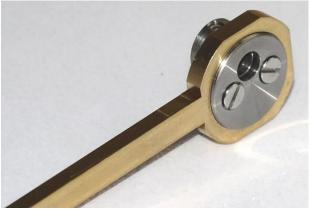
19. Connect the Valves with the Eccentric Rods using M2 10mm cap screws and lock each with a nut as shown in the following picture.
