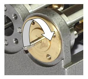
18. If not already assembled, put the Eccentric Wheels and Eccentric Wheel Plates together with the Eccentric Rods using the counter sunk M3 screws, as shown in the following picture. Then if not already in place, screw a 3mm grub/setscrew into the Eccentric Wheels which will be used to lock the wheels onto the Crank Shaft.
