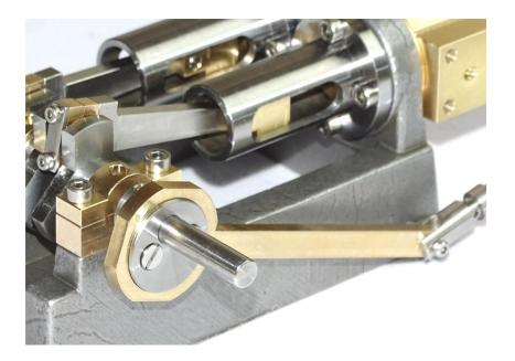
21. Insert the Valves into the Chests. The Chests can then be fixed to their respective Cylinders using 8 M3 18mm cap screws as shown in the following pictures.
