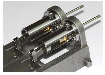
7. Remove the cap screws and the Main Bearing Uppers off the Base. Ensure these are later replaced in the same place and orientation as they are machined in pairs.
