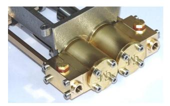
24. Screw the 2 Value Inlet Pipes into the remaining holes in the Chests (these stub pipe is used for connecting to an air source). The threaded holes in the chest are ¼" x 40 tpi ME which will accommodate the most common connection to a model steam boiler.
