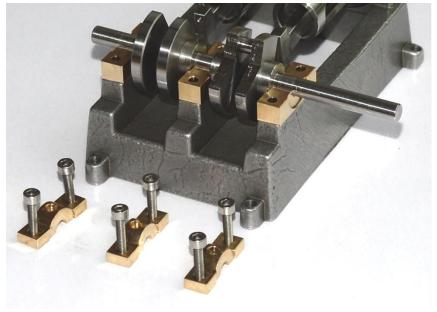
Place the Crank Shaft onto the Main Bearing Lowers and replace the Uppers, as shown in the following picture. Evenly and gradually tighten the 6 cap screws whilst rotating the shaft. This will ensure the bearings centre themselves properly on the shaft. Lubricate via the hole in the Upper bearings.
