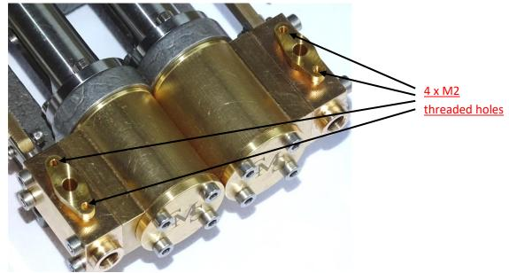
28. Place 2 cap screws in each of the remaining 2 Manifolds and ¼" brass locking nuts, as per the following picture.
