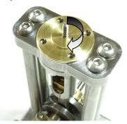
21. Put the Eccentric Wheel and Eccentric Wheel Plate together around the Eccentric Rod using the counter sunk M3 screws, as shown in the following pictures. Use the Crankshaft to ensure the parts are aligned and can rotate freely before fully tightening the screws. Then, if not already in place, screw a 3mm grub/setscrew into the Eccentric Wheel which will be used to lock the wheels onto the Crankshaft.
