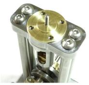
17. If not already in place, insert the 2 nylon piston rings into the slots in the piston and screw the Piston onto the Piston Shaft. Lock the shaft to the piston using an M3 nut tightened with a small pair of pliers or spanner – be careful not to damage the piston or shaft when tightening the nut.
