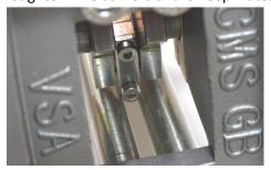
14. Screw the Packing Nut into the Cylinder Plate Inner.
