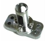
10. Check that none of the capscrews protrudes above the surface of the Top Plate. If any do remove the capscrew, file down and replace.
