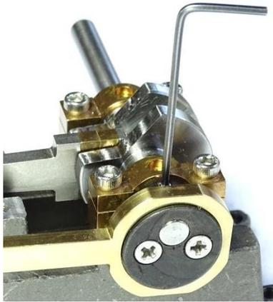
19. Screw the Inlet (stub) Pipe and the Chest Plug into the Chest. The pipe and plug can be reversed depending on if the chest is fed with steam/air from the top or bottom of the engine. The threaded holes in the chest are  $\frac{1}{4}$ " x 40 tpi ME which will accommodate the most common connection to a model steam boiler such as the Chiltern Model Steam boiler.
