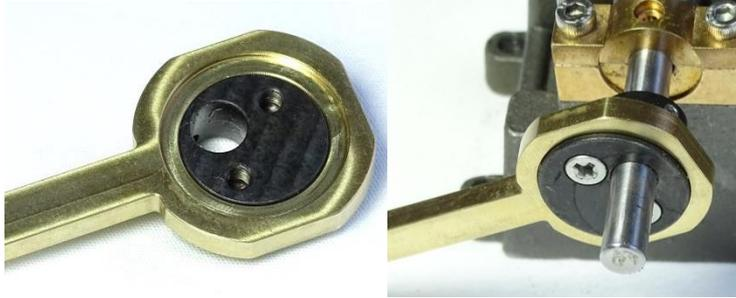
16. Connect the Valve with the Eccentric Rod using an M2 10mm capscrew and lock with a nyloc nut as shown in the following picture.
