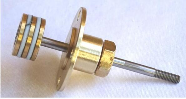
4. Screw an M3 nut onto the Piston Shaft and then the Shaft Parallel Spacer. Approximately 1mm of thread on the Piston Shaft should still then be visible. Lock the Shaft Parallel Spacer in place with the M3 nut with a 5.5mm spanner..
