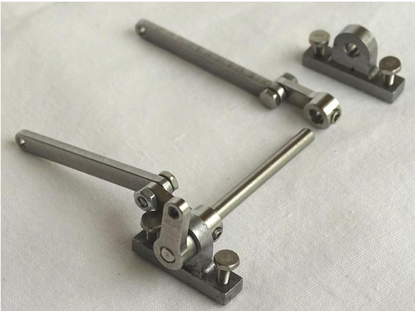
29. Check and cut to length the 4 M2 cap screws used to fix the Eccentric Level Shaft Bearings onto the Base by trial fitting them in place.
