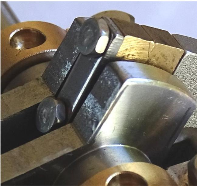
18. The Connecting Rod is fixed to the Beam using 2 Pivot Screws.
