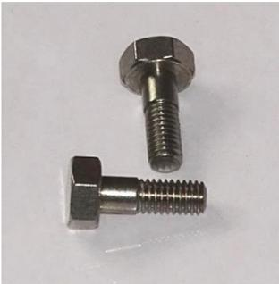
19. Screw the 2 Pivot Screws through the Connecting Rod holes into the threaded lugs on the Beam. The threaded lugs are tapped right through the Beam so that the 2 Pivot Screws can lock against each other in the middle when tightened. Turn the Crank Shaft to ensure the Beam/Connecting Rod can move freely.
