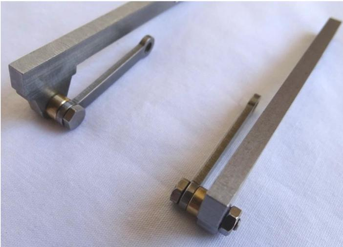
21. Push a 15mm cap screw through the other hole of the Parallel Link connected to the Column Arm, in the opposite direction of the cap screw holding the Parallel Link to the Column Arm.
