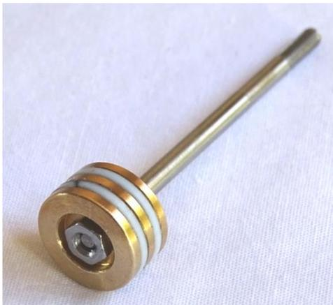
3. Screw the Packing Nut into the Cylinder Plate Inner and push onto the shaft as per the following picture.
