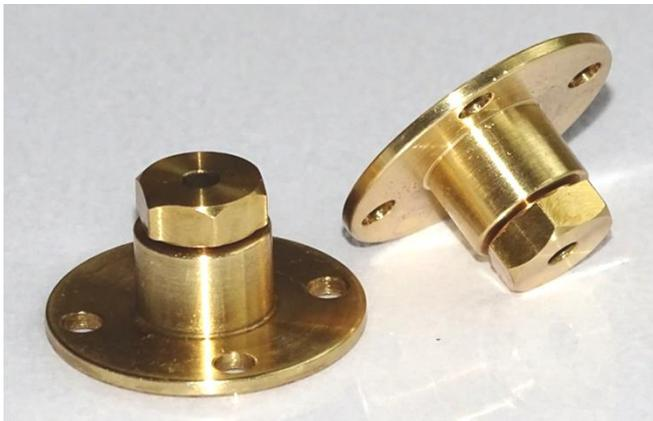
12. If it is planned to use high pressure steam - during final assembly, to improve the seal around the piston shaft, PTFE tape can be wrapped around the shaft and Packing Nut thread. When tightening the Packing Nut into the plate ensure the shaft can still move freely, that is, do not screw tight. Place one Cylinder Plate Inner/Packing Nut onto a Piston Shaft.
