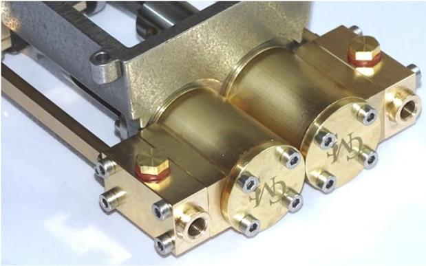
24. Screw the 2 Valve Inlet Pipes into the remaining holes in the Chests (these stub pipe is used for connecting to an air source). The threaded holes in the chest are  $\frac{1}{4}$ " x 40 tpi ME which will accommodate the most common connection to a model steam boiler.
