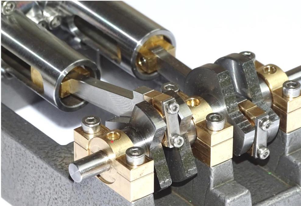
10. Check the sliders run smoothly in their tubes by rotating the crank. The tubes may need some lubrication to clean it out and ensure smooth operation.
