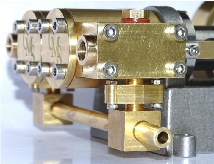
35. Lubricate the engine to ensure it operates freely.
