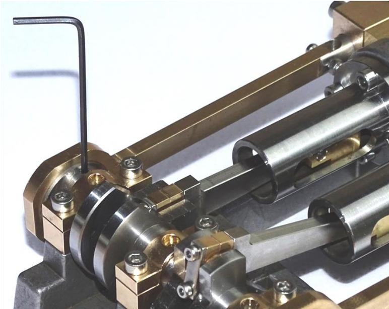
23. The steam inlets can be on top or bottom of the engine Chests. If, as in the following photos, the inlet is on top, screw the 2 Chest Plugs into the holes on the bottom of the Chests. PTFE tape or fibre washers can be used to seal the Chest Plugs if needed. NOTE: The RED Fibre washers are not now included.
