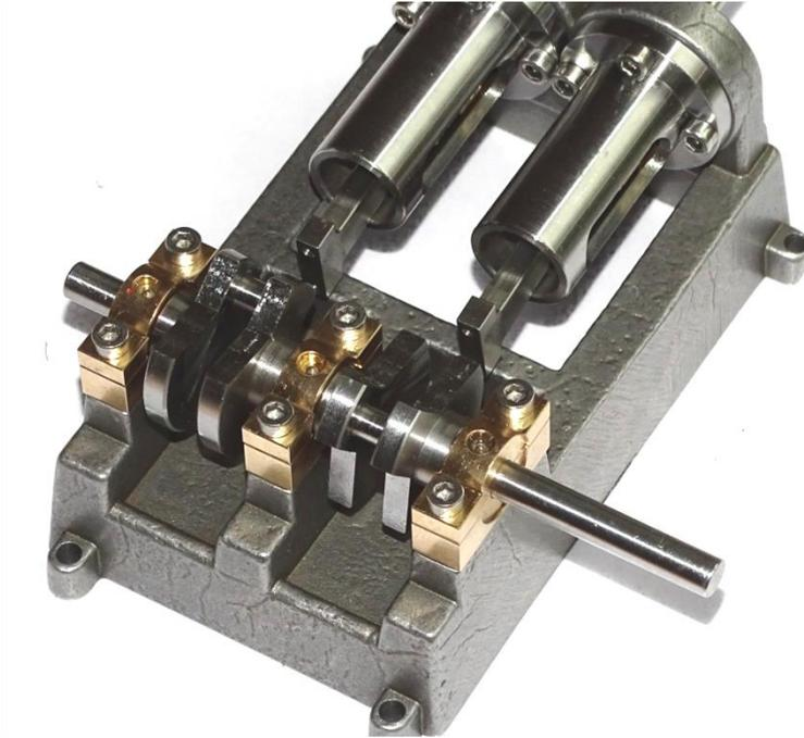
9. One side at a time, place the Connecting Rod Bearing halves and Keep around the Crank Shaft as shown in the following picture. Insert and tighten the cap screws evenly and gradually using the 1.6mm hex/allen key, rotating the connecting rod around the shaft to ensure the bearing halves locate centrally.
