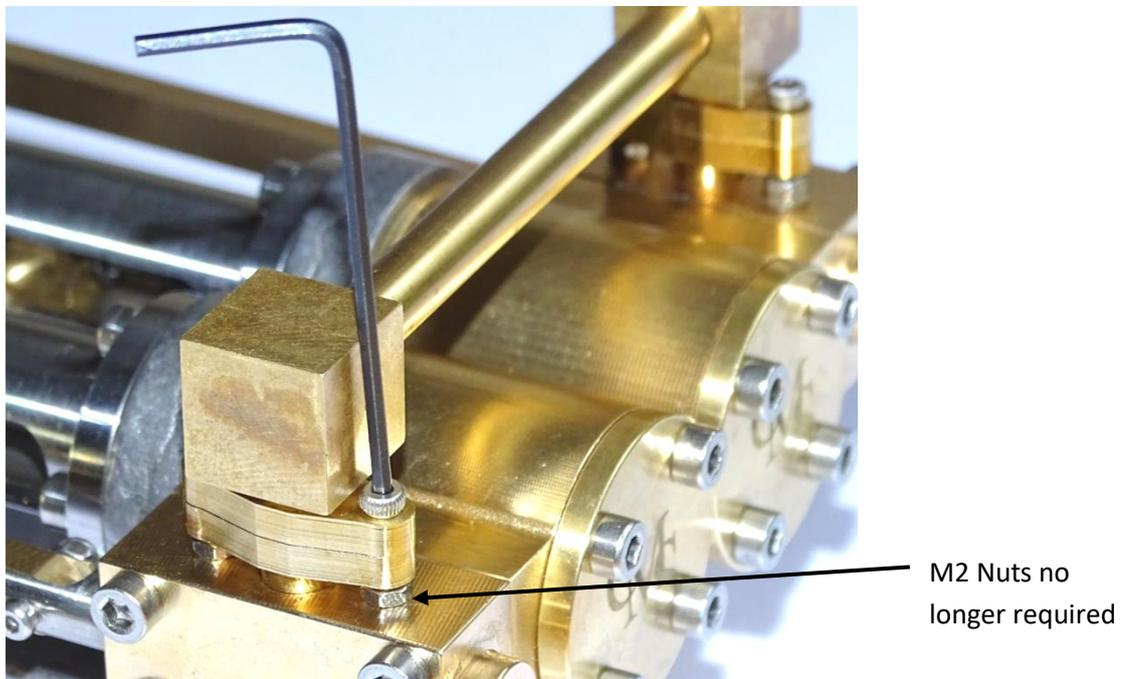
31. Some trial and error may be required to get the Manifolds to accurately mate together, i.e. screwing out or in the Link Pipe and/or Manifolds. Once aligned fix the Manifolds together using the 4 x M2 cap screws and tighten the 1/4" lock nuts.
