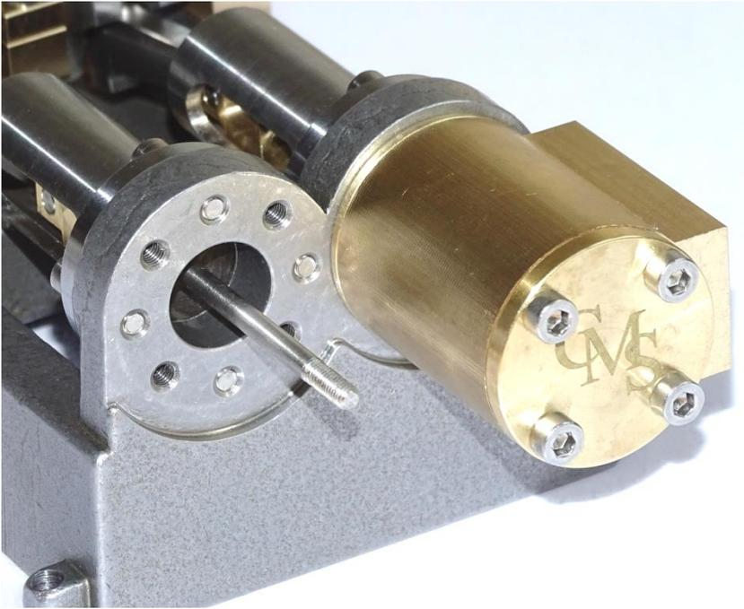
15. Before tightening the cap screws rotate the Crank Shaft to ensure the Piston can move freely in the Cylinder. There is some tolerance in the Cylinder and Cylinder Plate holes to allow them to be moved into a suitable position to allow free movement of the piston.
