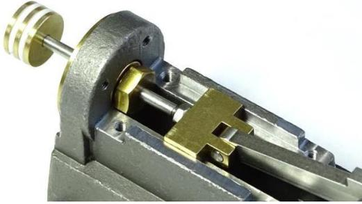
11. The Piston Shaft is locked to the Crosshead Slider using an M3 nut and a small pair of pliers or spanner. Usually it is not necessary but the Piston Shaft can be screwed into or out of the Crosshead Slider before locking in position to more accurately centralise the “throw” of the piston in the Cylinder.
