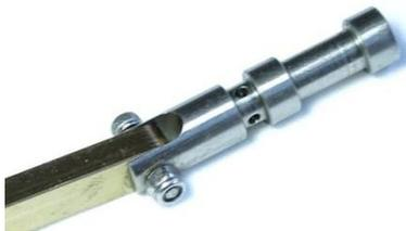
17. Push the Eccentric Wheel on to the short end of Crank Shaft and then insert the Valve into the Chest. The Chest can then be fixed to the Cylinder using 4 M3 18mm setscrews as shown in the following picture.
