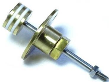
9. If it is planned to use high pressure steam - during final assembly, to improve the seal around the piston shaft, PTFE tape can be wrapped around the shaft and Packing Nut thread. When tightening the Packing Nut into the plate ensure the shaft can still move freely, that is, do not screw tight.
