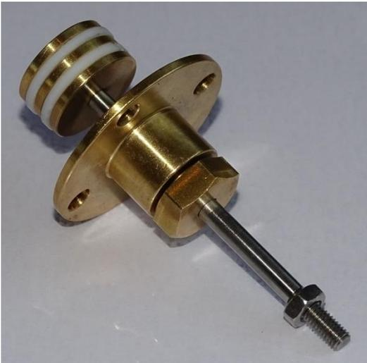
4. If it is planned to use high pressure steam - during final assembly, to improve the seal around the piston shaft, PTFE tape can be wrapped around the shaft and Packing Nut thread. When tightening the Packing Nut into the plate ensure the shaft can still move freely.
