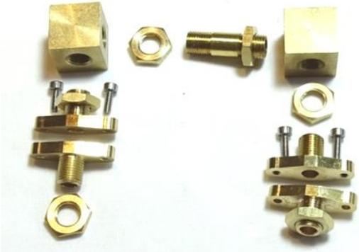
24. Screw the 2 Inlet Manifolds that have threaded holes into the remaining Chest inlet holes. Use the ¼" brass locking nuts to fix the Manifolds in position.
