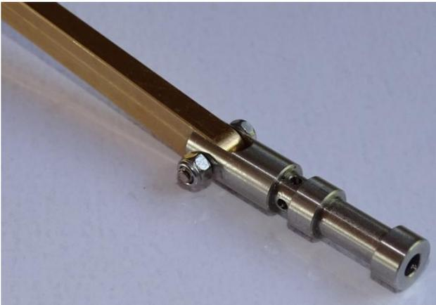
14. As per the following picture, push each Eccentric Wheel onto the longer end side of a Crank Shaft – the grub setscrew part of the Eccentric Wheel face the crank. Then push each Crank Shaft's longer end into the Flywheel hub. Ensure the 4 grub setscrews (2 each side) are in place in the Flywheel but don't tighten at this stage.
