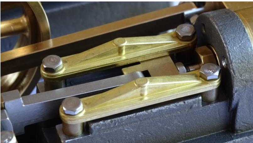
22. Screw the Chest Plug with fibre washer into the Chest top or bottom. The plug can be reversed depending on if the chest is fed with steam/air from the top or bottom of the engine. The threaded holes in the chest are  $\frac{1}{4}$ " x 40 tpi ME which will accommodate the most common connection to a model steam boiler such as the Chiltern Model Steam boiler.
