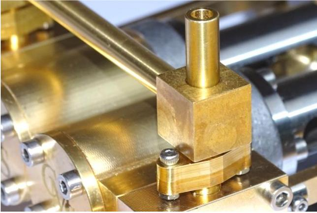
34. NOTE: The tee can be reoriented to allow an horizontal inlet direction rather than top/vertical as show in the above photo and as mentioned earlier the manifold can be installed on the bottom of the Chest/engine with Chest Plugs on the top.
