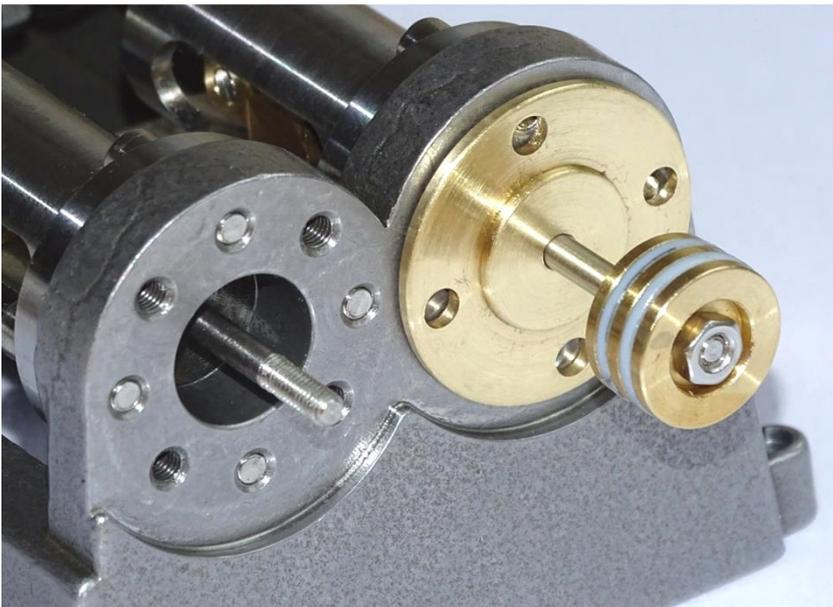
14. Place a Cylinders onto the Cylinder Plate Inner and Piston and place the Cylinder Plate End on top of that. Align the holes in the Cylinder Plates and Cylinders with the threaded holes in the Base and screw in the M3 45mm cap screws as shown in the following picture.
