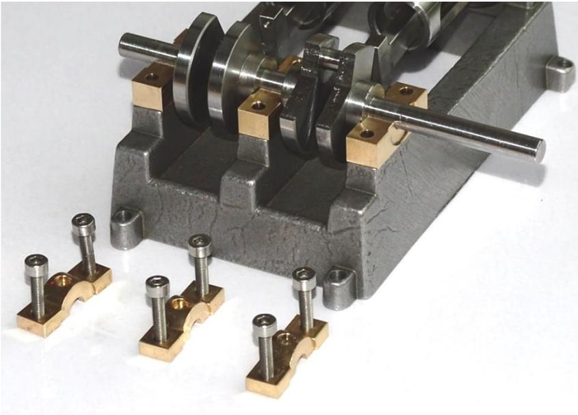
8. Place the Crank Shaft onto the Main Bearing Lower and replace the Uppers, as shown in the following picture. Evenly and gradually tighten the 6 cap screws whilst rotating the shaft. This will ensure the bearings centre themselves properly on the shaft. Lubricate via the hole in the Upper bearings.
