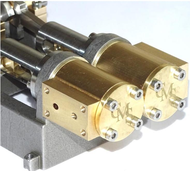
17. If after tightening the Cylinders the engine does not turn over freely try rotating the Cylinder Plates Inner by 90°. Similarly try refitting the Slides/Connecting Rods and its bearings the other way up.
