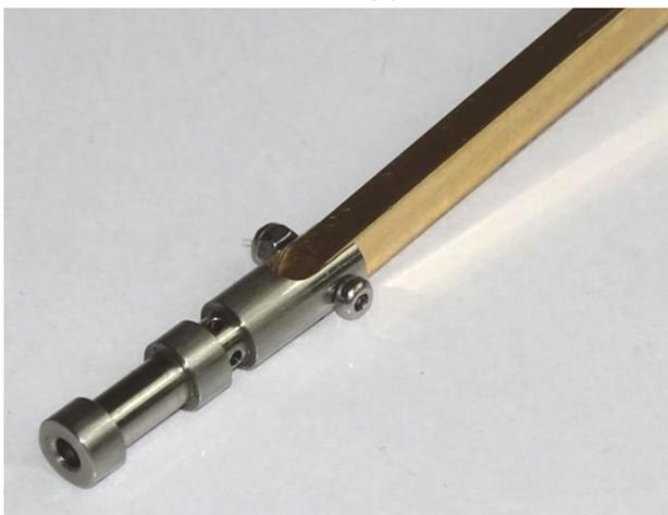
20. Push the 2 Eccentric Wheels on to the 2 ends of Crank Shaft, don't tighten the grub/setscrews yet.
