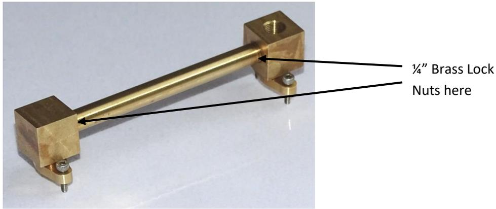
30. Place the Inlet Manifold/Connector subassembly on the Manifolds already installed on the Chests, aligning the Manifold holes to allow the cap screws to go through.
