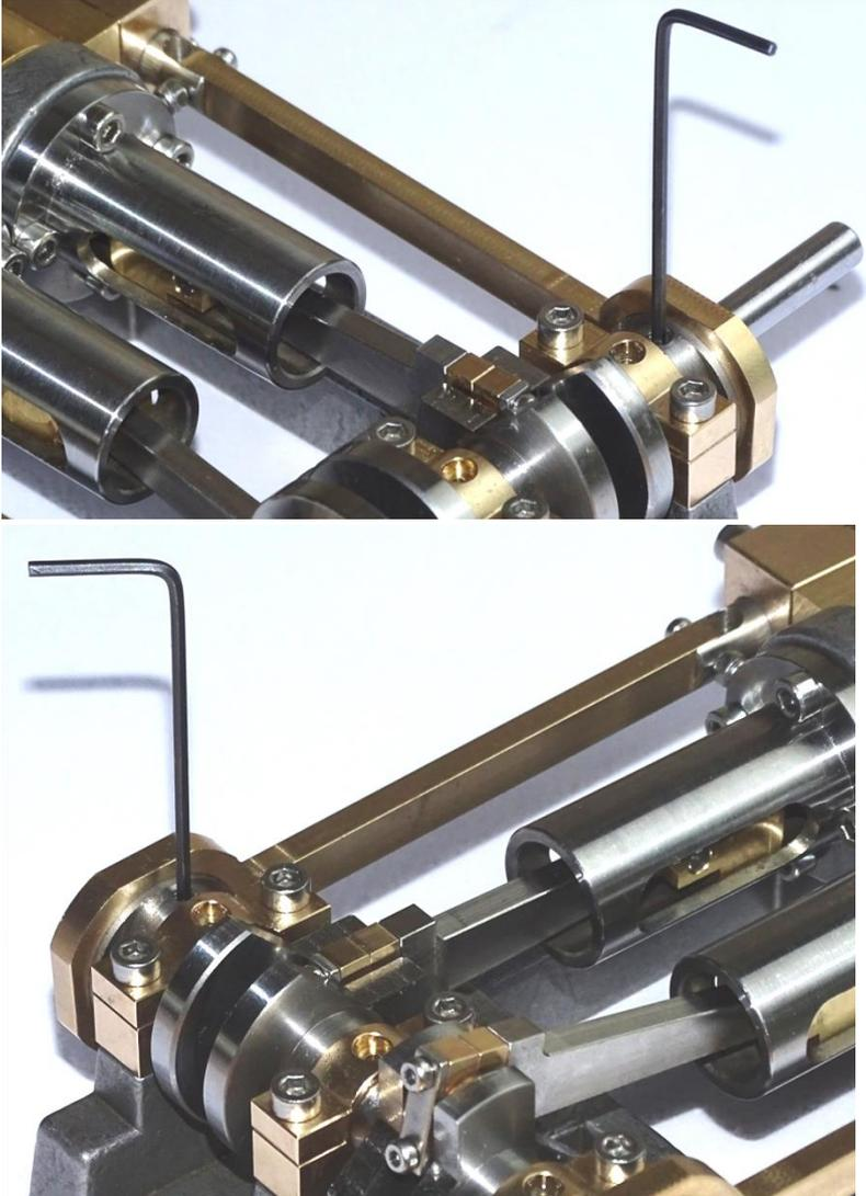
23. The steam inlets can be on top or bottom of the engine Chests. If, as in the following photos, the inlet is on top, screw the 2 Chest Plugs into the holes on the bottom of the Chests. PTFE tape or fibre washers can be used to seal the Chest Plugs if needed. NOTE: The RED Fibre washers are not now included.
