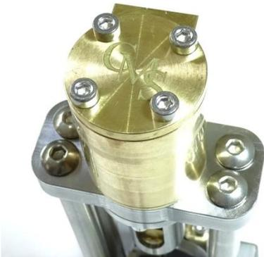
19. Before tightening the 40mm capscrews rotate the Crank Shaft to ensure the Piston can move freely in the Cylinder. There is some tolerance in the Cylinder and Cylinder Plate holes to allow them to be moved into a suitable position to allow free movement of the piston. Then gradually tighten the 40mm capscrews.
