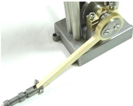
24. Insert the Valve into the Chest. The Chest can then be fixed to the Cylinder using 4 M3 18mm capscrews.
