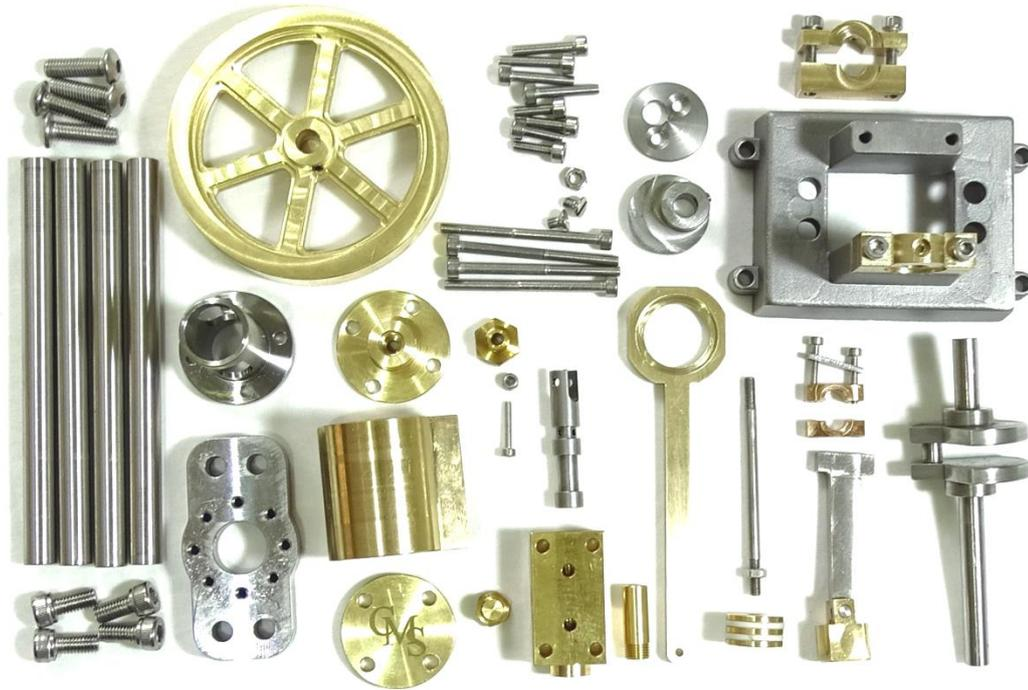
2. Remove the M3 capscrews and the Main Bearing Uppers off the Base Plate. Ensure these are later replaced in the same place and orientation as they are machined in pairs.
