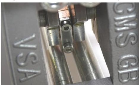
14. Screw the Packing Nut into the Cylinder Plate Inner.
