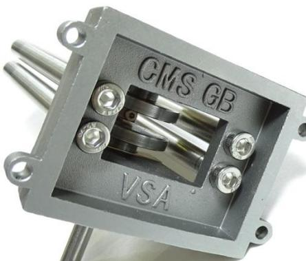
9. Fix the Slider Tube to the Top Plate using the 10mm M3 capcrews. NOTE: Capcrews as supplied may need to be shortened.
