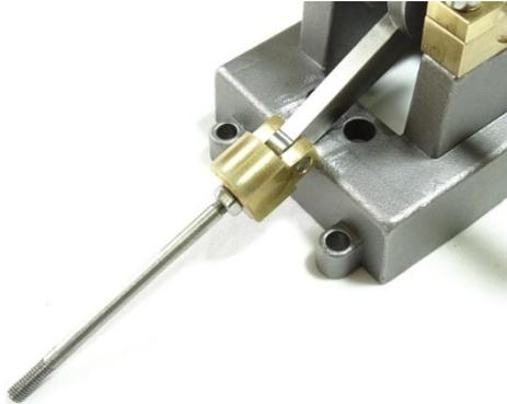
7. NOTE: Usually it is not necessary but the Piston Shaft can be screwed out of the Slider to more accurately centralise the “throw” of the piston in the Cylinder.
