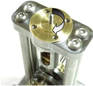
21. Put the Eccentric Wheel and Eccentric Wheel Plate together around the Eccentric Rod using the counter sunk M3 screws, as shown in the following pictures. Use the Crankshaft to ensure the parts are aligned and can rotate freely before fully tightening the screws. Then, if not already in place, screw a 3mm grub/setscrew into the Eccentric Wheel which will be used to lock the wheels onto the Crankshaft.
