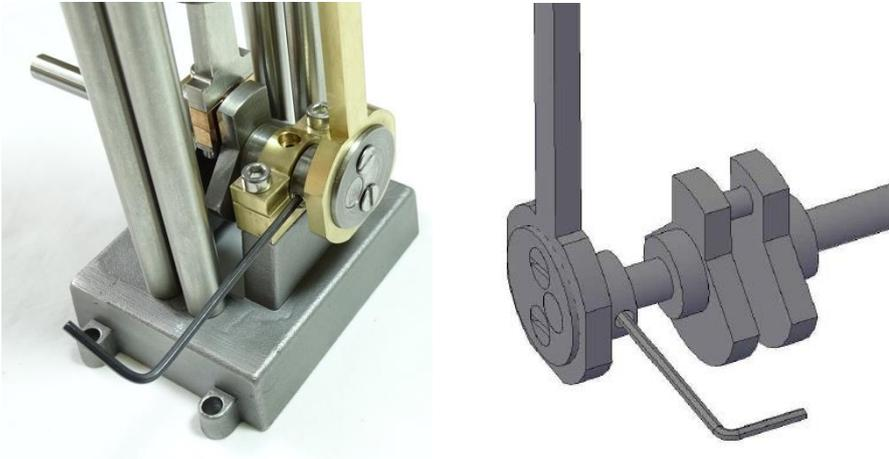
26. Screw the Chest Plug and Inlet/Outlet Pipe, used for testing on compressed air, into the Chest. The Chest Plug can be on either side of the Chest depending on which side the steam pipe from the boiler needs to be connected.
