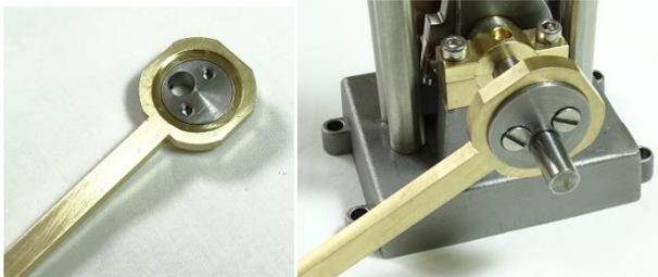
22. Connect the Valve with the Eccentric Rod using a M2 10mm capscrew and nyloc nut as shown in the following picture. The nut should be very slightly loose to ensure free movement of the Valve on the Eccentric Rod.
