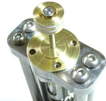
18. Place the Cylinder over the Piston and the End Plate on top of the Cylinder. Then loosely screw them in place using the 40mm M3 capscrews.
