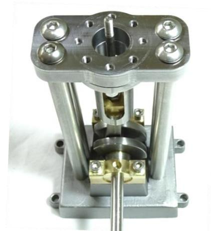
12. Gradually tighten all 8 M5 stop and button capcrews whilst rotating the Crankshaft.
