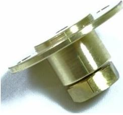
15. If it is planned to use high pressure steam - during final assembly, to improve the seal around the Piston Shaft, a small amount of PTFE tape can be wrapped around the Shaft and pushed into place with the Packing Nut. When tightening the Packing Nut into the plate ensure the Shaft can still move freely.
