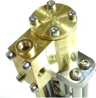
25. Rotate the Eccentric Wheel and Shaft until they are 90° to each other, as shown in the following picture. NOTE: When the Eccentric Wheel is fixed 180° to the position shown the engine will run in the opposite direction.
