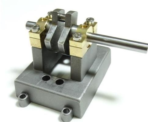
4. Remove the M2 screws holding the connecting rod bearing halves to the connecting rod and place them around the crank shaft as shown in the following picture. Insert and tighten the screws evenly and gradually, rotating the connecting rod around the shaft to ensure the bearing halves locate centrally.
