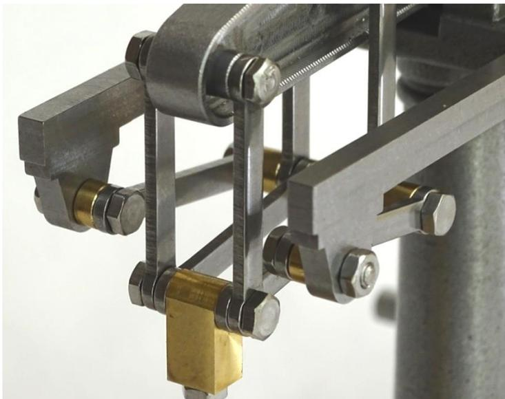
27. Fix the 2 Eccentric Links to the 2 Eccentric Levers using 2 M2 cap screws as per the following picture. The holes in the Eccentric Levers are threaded, so tighten the M2 cap screws then back off half a turn before using an M2 nut to lock the cap screw. Eccentric Links need to be able to freely rotate but not be too loose. The M2 cap screws can be shortened neatly during final assembly.
