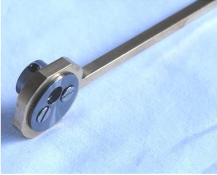
34. Push the Eccentric Wheel onto the long end of the Crank Shaft and lock into position on the shaft with the grub/setscrew as per the following picture – this is the Valve timing. NOTE: If the Eccentric Wheel is positioned 180 degrees to the Crank to that shown in the picture the engine will run in the reverse direction.
