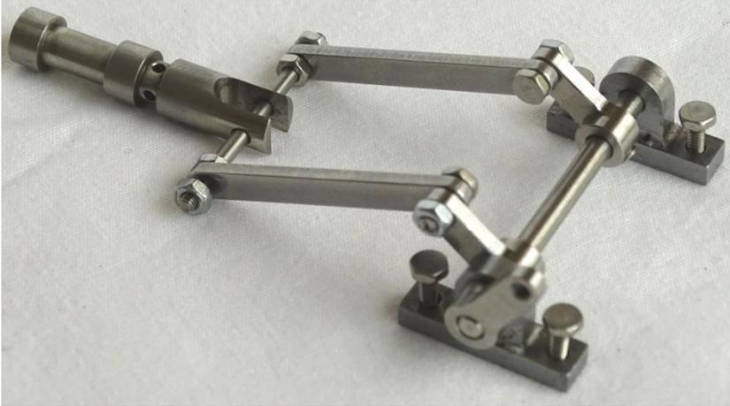
31. Push the Valve into the Chest and screw the Eccentric Level Shaft Bearings to the Base using the 4 M2 cap screws.
