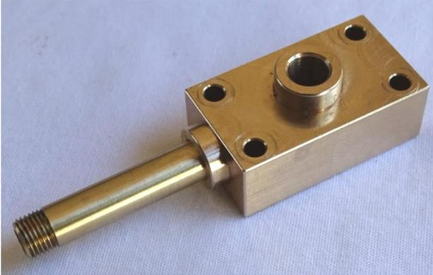
8. Using 4 18mm cap screws and as earlier optional brass washers, fix the Chest onto the Cylinder with the Outlet Pipe pointing down through the hole in the Base.
