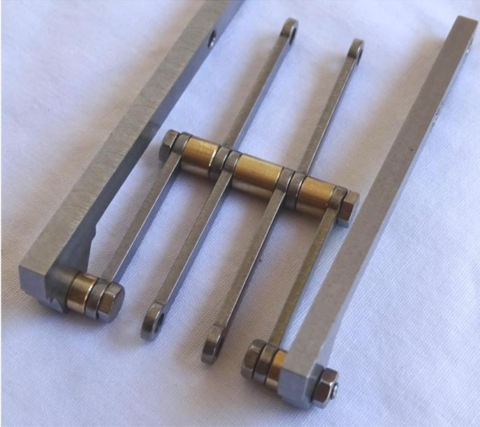
22. The Parallel Spacer Centre is threaded through so that the 2 cap screws are locked in place by tightening them against each other inside the Parallel Spacer Centre. When the 2 cap screws are tightened it is important to ensure that all the Parallel Links can still move freely but are not overly loose. To achieve this it will probably be necessary to file the cap screws to length – do this gradually by testing and refitting a few times.
