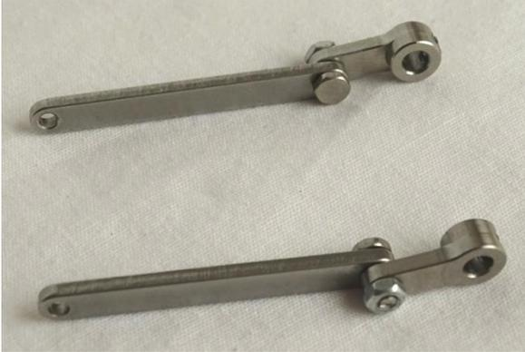
28. Push an Eccentric Lever/Link onto the Eccentric Lever Shaft, then an Eccentric Lever Shaft Bearing on that end, then the third Eccentric Lever (not connected to an Eccentric Link), as per the following picture. If not already in place, fit the short grub/set screws in the Eccentric Levers but just tighten the third Eccentric Lever to the shaft at this stage.
