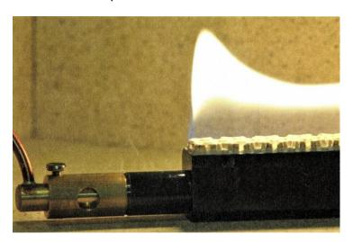
To get the burner running correctly loosen the locking screw and *very slightly* move the jet carrier out of the burner tube, tighten the screw, light, wait 30 seconds and observe the flame. Turn off the gas and allow the burner to cool before repeating the process. The burner is set correctly when there are *little blue jets* dancing on the ceramic and (almost) no yellow flame above them.
