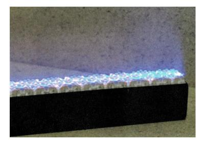
The burner can now be installed beneath the boiler cylinder when fine tuning may be necessary.
