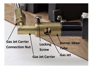
The gas jet size installed in the carrier is No. 8.
