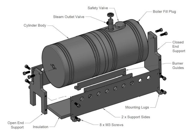
Gradually tighten each screw ensuring the supports are not twisted and sits flat on a mounting board (customer supplied).
