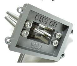
9. Fix the Slider Tube to the Top Plate using the 10mm M3 capcrews. NOTE: Capscrews as supplied may need to be shortened.
