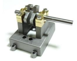
4. Remove the M2 screws holding the connecting rod bearing halves to the connecting rod and place them around the crank shaft as shown in the following picture. Insert and tighten the screws evenly and gradually, rotating the connecting rod around the shaft to ensure the bearing halves locate centrally.
