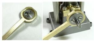
22. Connect the Valve with the Eccentric Rod using a M2 10mm capscrew and nyloc nut as shown in the following picture. The nut should be very slightly loose to ensure free movement of the Valve on the Eccentric Rod.
