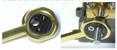
16. Connect the Valve with the Eccentric Rod using an M2 10mm capscrew and lock with a nyloc nut as shown in the following picture.
