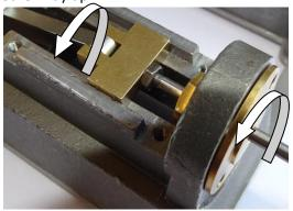
15. Put the Eccentric Wheel and Eccentric Wheel Plate together with the Eccentric Rod loosely using the counter sunk M3 screws. Push the sub-assembly onto the crank shaft to ensure the wheel and plate are aligned before tightening the screws, as shown in the following picture. Then if not already in place, screw a 3mm grub/setscrew into the Eccentric Wheel which will be used to lock the wheel onto the Crank Shaft.
