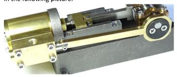
18. Set the angle of the Eccentric Wheel to the Crank as shown in the following picture and on the Assembly drawing. Tighten the grub/setscrew.
