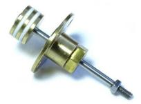
9. If it is planned to use high pressure steam - during final assembly, to improve the seal around the piston shaft, PTFE tape can be wrapped around the shaft and Packing Nut thread. When tightening the Packing Nut into the plate ensure the shaft can still move freely, that is, do not screw tight.
