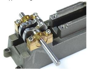
4. Remove the screws holding the connecting rod bearing halves to the connecting rod and place them around the crank shaft as shown in the following picture. Keeping the Bearing Keep in place, insert and tighten the screws evenly and gradually, rotating the connecting rod around the shaft to ensure the bearing halves locate centrally.
