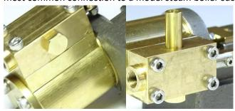
20. Fit the 2 Slider Caps together with the Slider Cap Spacers onto the Vertical Base Top using M3 capscrews.
