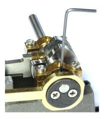
19. Screw the Inlet (stub) Pipe and the Chest Plug into the Chest. The pipe and plug can be reversed depending on if the chest is fed with steam/air from the top or bottom of the engine. The threaded holes in the chest are ¼" x 40 tpi ME which will accommodate the most common connection to a model steam boiler such as the Chiltern Model Steam boiler.
