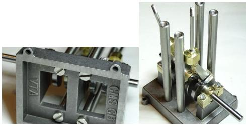
8. Fix the Slider Tubes to the Top Plate using the 12mm M3 capcrews.
