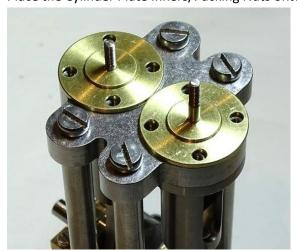
16. If not already in place, insert the 2 nylon piston rings into the slots in the piston and screw the Pistons onto each Piston Shaft. Carefully lock the shafts to the pistons using an M3 nut tightened with a spanner or small pair of pliers.
