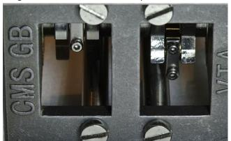
13. Screw each Packing Nut into the Cylinder Plate Inners.
