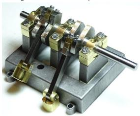
5. Screw the M3 nut onto each Piston Shaft on the longer threaded end. The end of the shaft with the shorter thread is for the Piston.
