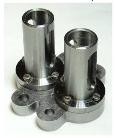
9. Check that none of the capscrews protrudes above the surface of the Top Plate. If any do remove the capscrew, file down and replace.
