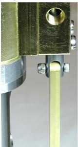
24. Screw the Chest Plugs and Inlet (stub) pipes into the Chests. The threaded holes in the chest are ¼" x 40 tpi ME which will accommodate the most common connection to a model steam boiler.
