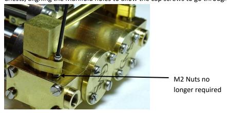
31. Some trial and error may be required to get the Manifolds to accurately mate together, i.e. screwing out or in the Link Pipe and/or Manifolds. Once aligned fix the Manifolds together using the  $4 \times M2$  cap screws and tighten the  $\frac{1}{4}$ " lock nuts.
