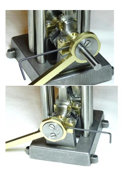
23. Insert the Valves into the Chests. The Chests can then be fixed to their respective Cylinders using 4 M3 18mm setscrews.
