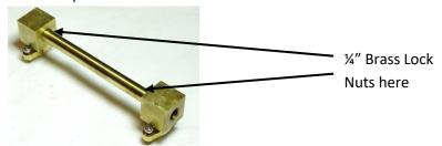
30. Place the Inlet Manifold/Connector subassembly on the Manifolds already installed on the Chests, aligning the Manifold holes to allow the cap screws to go through.
