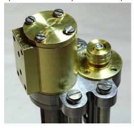
18. Before tightening the 45mm capscrews rotate the Crank Shaft to ensure the Piston can move freely in the Cylinder. There is some tolerance in the Cylinder and Cylinder Plate holes to allow them to be moved into a suitable position to allow free movement of the piston. Then gradually tighten the 45mm capscrews. Repeat for the second Cylinder.
