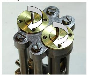
20. Put the Eccentric Wheels and Eccentric Wheel Plates together with the Eccentric Rods loosely using the counter sunk M3 screws. Slide the Eccentric onto the crank shaft to ensure the wheel and plate aligns before tightening the screws, as shown in the following pictures. Then if not already in place screw a 3mm grub/setscrew into the Eccentric Wheels which will be used to lock the wheels onto the Crank Shaft.
