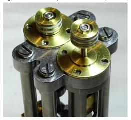
17. One at a time, place the Cylinders over the Pistons and the End Plates on top of the Cylinders. Then loosely screw them in place using the 45mm M3 capscrews.
