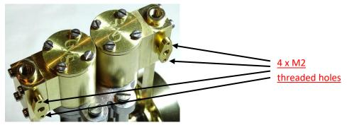
28. Place 2 cap screws in each of the remaining 2 Manifolds, as per the following picture.
