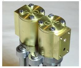
19. If after tightening the Cylinders the engine does not turn over freely try rotating the Cylinder Plates Inner by 90°. Similarly try refitting the Slides/Connecting Rods and its bearings the other way around.
